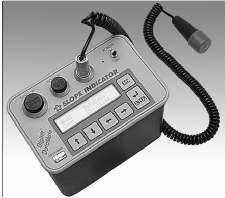
Simple to operate, the compact Digitilt DataMate runs 16 hours on one charge, stores up to 320 surveys, and transfers data to a PC for processing.
